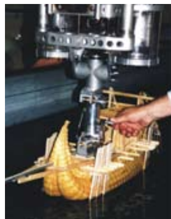
The positions of pre-Egyptian side-swords were calculated exactly according to their positions and tested positively in Kiel University's flow channel.
